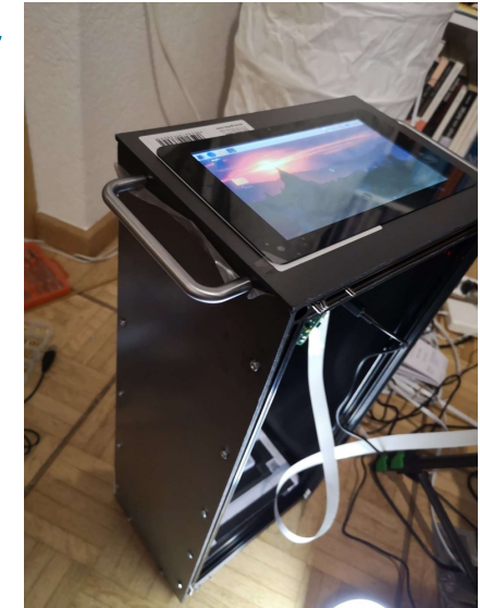
New hardware prototype (with touch screen and Raspberry Pi 4 Model B) for the Swiss Armed Forces
